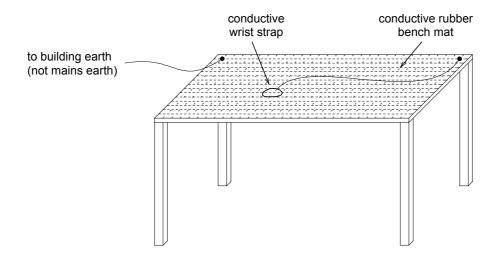
Figure 1.2 Typical Anti-static Bench Set-up
