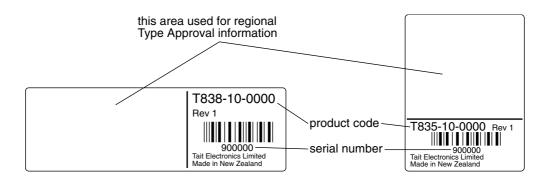
Figure 1.1 Typical Product Code & Serial Number Labels
